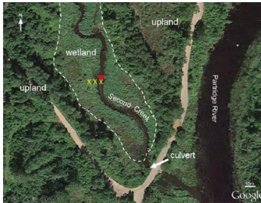
Figure 1: Second Creek Study Site. Yellow X's indicate the location of each temperature probe and collocated piezometer. From west to east, each location is referred to as the “west wetland”, “west streambed”, and the “center streambed”.
